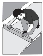
Compact the soil with a garden roller and then spread the sand with a rake and level it by scraping and tamping with a length of timber. To support heavier loads, or if the soil is composed of clay or peat, lay a subbase of firmly compacted hardcore (broken bricks or crushed stone) to a depth of 75 to 100mm before spreading the sand to level the surface. If you plan to park vehicles on the paving, increase the depth of hardcore to 150mm.
