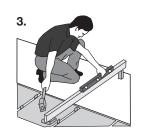
Check the alignment. Gauge the slope across the paving by setting up datum pegs along the high side. Drive them into the ground until the top of each corresponds to the finished surface of the paving, and then use a straight edge with a packing piece under one end to check the fall on the slabs.
