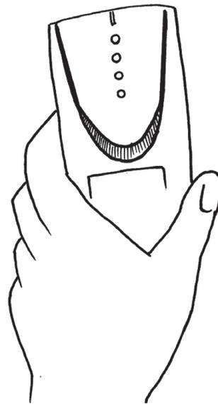
**Fig 1.** Electronic stud finder that beeps or flashes when it passes over wall studs or ceiling joists
