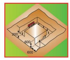
Put pegs in the bottom of the trench, about 1,5m apart and 200mm high. This will mark the depth of the concrete. Steps in the base should be the same height as a brick course. All pegs must be completely level.
