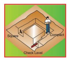
When digging is complete, to a depth of  $\pm 600$ mm, ensure the sides are plumb and the bottom level.
