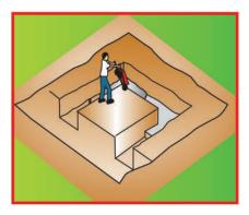
After mixing concrete pour into the foundation starting from one end. Keep level to the height of the pegs. Pour all concrete in one day.
