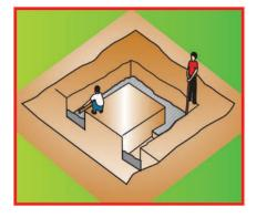
Level the concrete to the pegs and ram down to remove air spaces. Leave to set for **3 days** before building.
