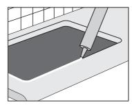
If the sink came with a rubber seal, attach it to the lip or, alternatively, use silicone. It is vital to ensure the edge has a watertight seal as it will affect the integrity of the worktop.
