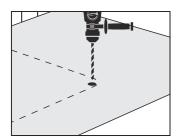
Drill an access point for the jigsaw blade with a 12mm drill or auger bit just inside the lip line.
