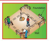
Mark the line of foundation on the ground with a spade, using the foundation lines as a reference. This can also be done using a line of cement to mark the foundation position.
