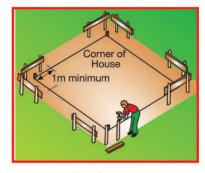
After marking out the walls of the house, put pegs in the ground 1 meter away from the house marking. Nail a piece of wood horizontally across the pegs. This will be used to mark the foundations.
