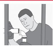
With plastic pipes, it is easy to correct a mistake. Simply cut out the problem section, correct the mistake and reassemble the joint with a coupling. Then cement the parts together.
