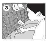
Remove any remaining sealant residue and grime with a tub and tile cleaner and a non-abrasive sponge.
