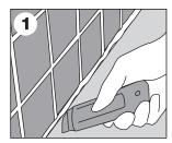
Push a utility knife in all the way under both edges of the old sealant bead to release its grip. Don't pry the sealant with the knife because you could break off the blade.
