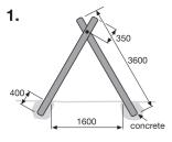
Make two A frame supports as shown. Drill 15mm holes 350mm from the ends of each of the 3600mm long poles. Take two of the poles and join them together with the threaded bar. Cut a length of threaded bar (350mm) and secure with washers and nuts. Do the same to the other pair of poles.
