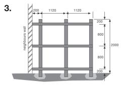
Insert three 76 x 76mm timber posts in the holes, 2450mm long. The length above ground level should be  $\pm$  2000mm. Level the posts and screw a 50 x 76mm batten across the three posts, 200mm above ground level. Use 76mm galvanized wood screws for this, two per fixing. The end of the batten can be fixed to the neighbor's fence with an aluminum angle cleat.
