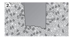
Attach 76mm nails to that section of the post that will be covered by concrete. Three per post. This will secure the posts in the concrete and make it difficult for them to be pulled out.
