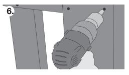
Using a cordless drill, fix 25 x 100 x 2000mm fence panels to the horizontal battens using 38mm galvanized screws. Two per fixing. The panels must be butted up against each other. Make sure that the top of the fence panels are in a straight line. Use a builders line to check this.
