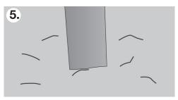
Fill holes with concrete and leave to set for 24 hours. For this job, premix concrete can be purchased in bags. Use one bag per hole.
