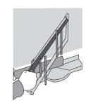
To cut a dado or picture rail you will need a mitre block and tenon saw or a mitre saw. When joining two pieces at a corner, mitre the ends to make a perfect 90° angle. Check each corner using a square. If not square, you will have to make adjustments to the mitre.
