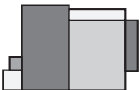
Divide an irregular shape into a series of squares and rectangles for the approximate area.
