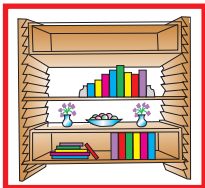
Cutting notches continuously to provide a shelf adjustment about every \pm 25\text{mm} .
